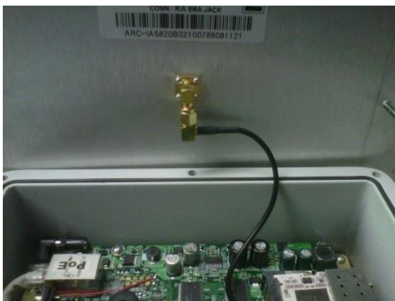
Inside view without Attenuator inside view with Attenuator Installed
