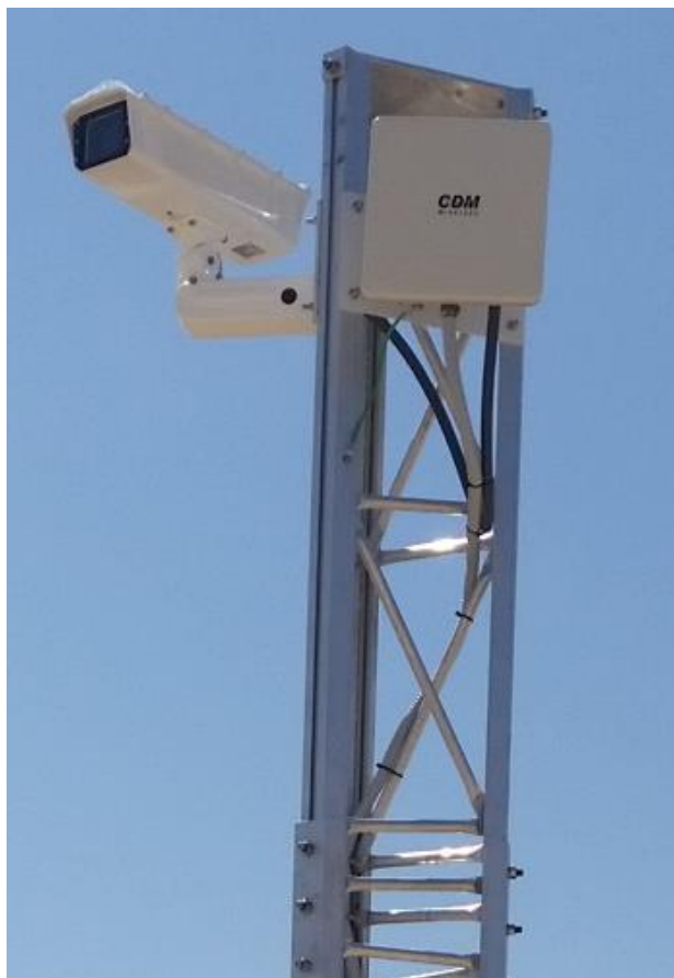
Properly oriented CDM Wireless Unit with integrated panel
