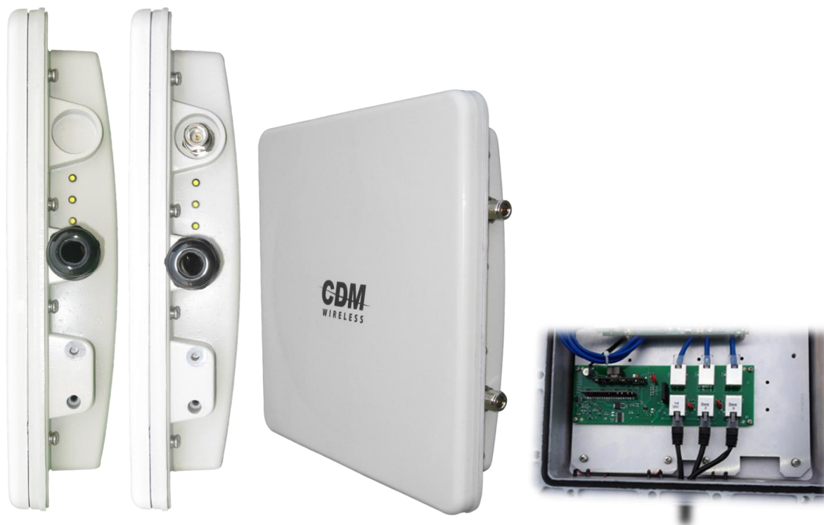
Figure 3a. Internal & External port connections
